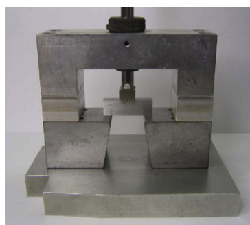
Fig. 11. Illustration of one of the test configurations to determine crack initiation and arrest micro fracture toughness of single crystal iron as a function of temperature, and example results for two crystal orientations.
